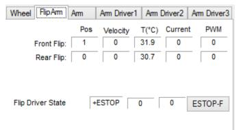
"FlipArm" tag will display all the information about the front/rear flip arm motors and the state of the flip arm motor driver board.
