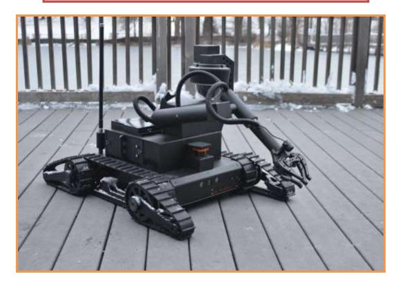
\*Shown with Options: Manipulator Arm, PTZ Camera, Laser Scanners, On-board Computer and Extended **Battery Packs**
