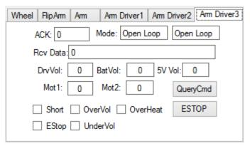
"Arm Driver3" tab will display motor driver 3 state (for optional pan unit).
